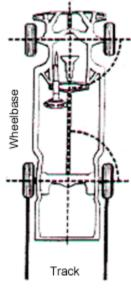
The side to side distance between the centerline of the tires on an axle is called track. The distance between the centerline of the front and rear tires is called wheelbase. If the vehicle is in proper alignment, the wheels will roll in a line that is parallel with the vehicle's geometric centerline.
