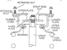
However, these components wear over time and with a thorough inspection a proper recommendation can be made. The bearing is located on the bottom of the strut mount and is not serviceable. Defective bearing will require replacement of the entire strut mount.
