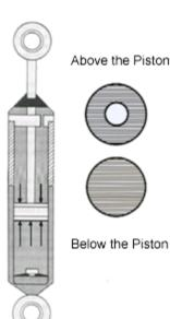
aeration reduced, the shock is able to react faster and more predictably, allowing for quicker response time and helping keep the tire firmly planted on the road surface.
