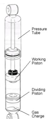
The area below the dividing piston is pressurized to about 360 psi with nitrogen gas. This high gas pressure helps support some of the vehicle's weight. The oil is located in the area above the dividing piston.
