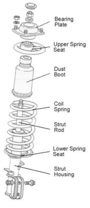
The top of the strut is connected to the vehicle body through the **upper strut mount**, in some cases called a**bearing plate**. This bearing plate allows the strut to pivot as the wheels are turned. It must be flexible enough to handle slight angle changes and dampen movement of the upper end of the strut. This mount or bearing plate transfers vehicle load to the strut and spring, making the upper mount/bearing plate the load carrier and the lower ball joint the follower.
