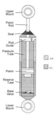
with the pressure tube and allows the piston to move freely inside. The **seal** keeps the hydraulic oil inside and contamination out.
