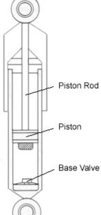
Let's start our discussion of shock absorbers with one of very important point: despite what many people think, conventional shock absorbers do not support vehicle weight. Instead, the primary purpose of the shock absorber is to control spring and suspension movement. This is accomplished by turning the kinetic energy of suspension movement into thermal energy, or heat energy, to be dissipated through the hydraulic fluid.
