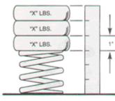
Spring rate, sometimes referred to as deflection rate, is used to measure spring strength. It is the amount of weight that is required to compress the spring 1 inch. For example: If it takes 100 lbs. to compress a spring 1inch, it would take to 200 lbs. to compress the spring 2 inches.
