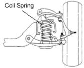
The diameter and length of the wire determine the strength of a spring. Increasing the wire diameter will produce a stronger spring, while increasing its length will make it more flexible.
