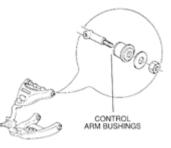
maintain the lateral and vertical location of the control arm pivot points, maintain dynamic wheel alignment, reduce transmitted noise, road shock, and vibration, while providing resistance to suspension movement.
