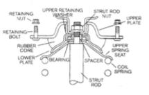
rubber bushing is cracked, torn, or the bearing is binding or seized, the strut mount requires replacement.
